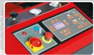
Inverter - Digital Control Panel
