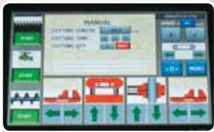
Inverter - PLC Control Panel
