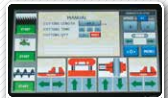
Inverter - PLC Control Panel
