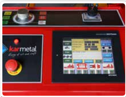
PLC Control Panel - Inverter
