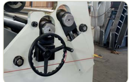
Kollu Alt Top / Hidrolik Arka Top Hareketi Manual Bottom Roll / Hydraulic Back Roll Movement
