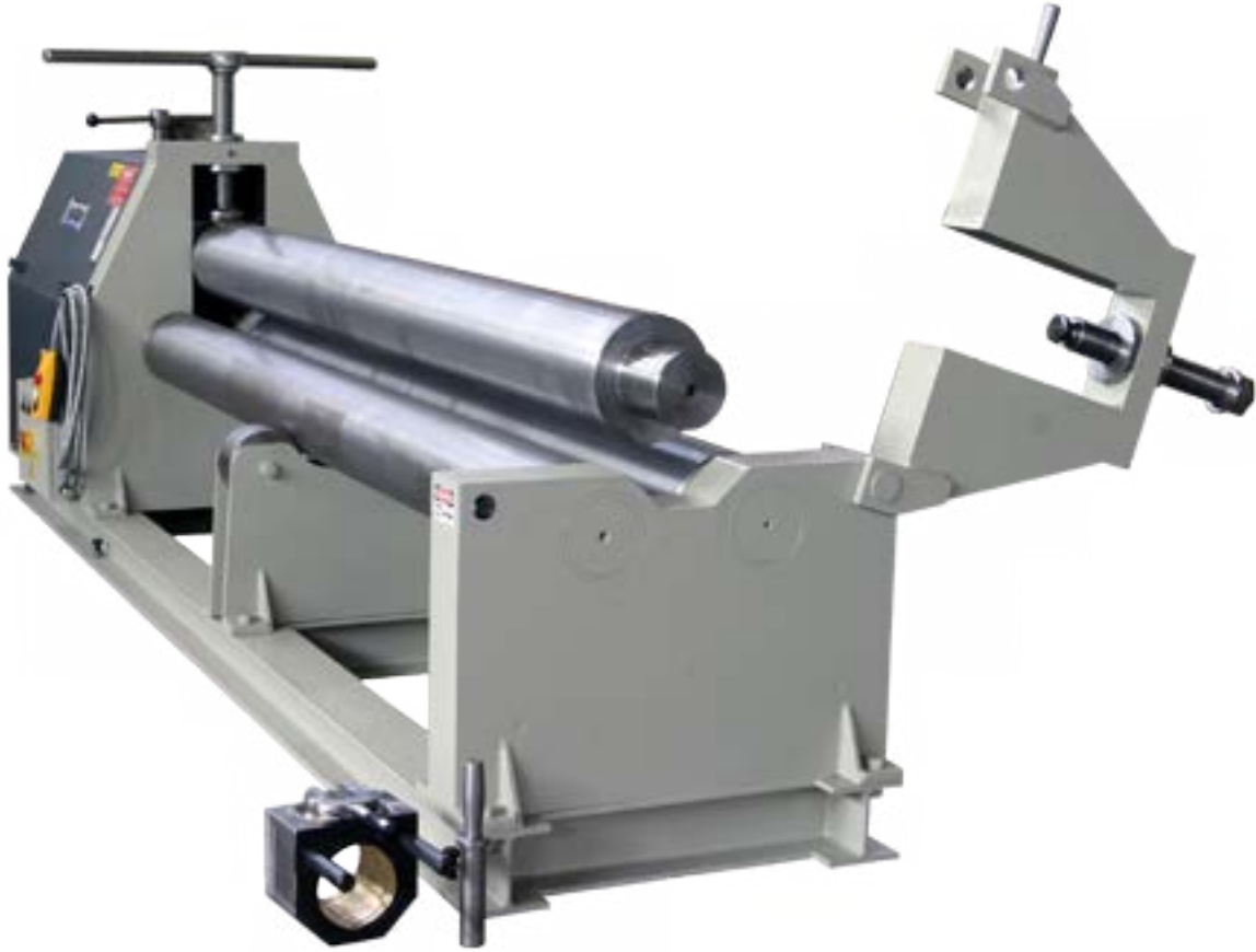
Model IS Manuel (kollu) üst top hareket Manual by hand top roll movement
