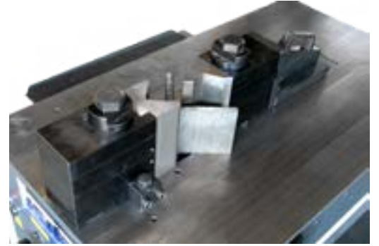
Standart Abkant Kalıbı V-Pressbrake Punch & Die included as standard
