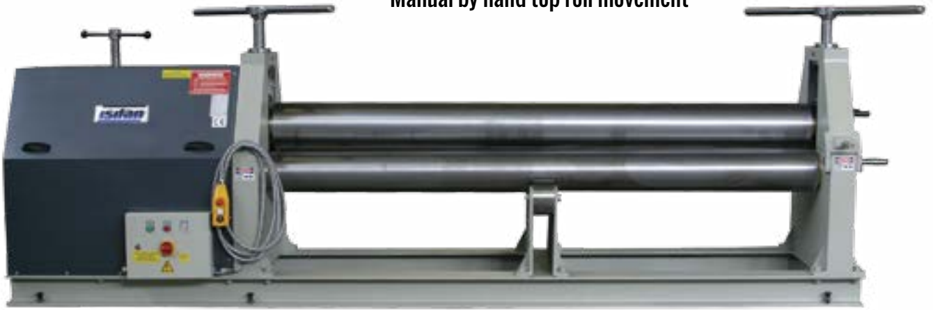
Model IS Manuel (kollu) üst top hareket Manual by hand top roll movement
