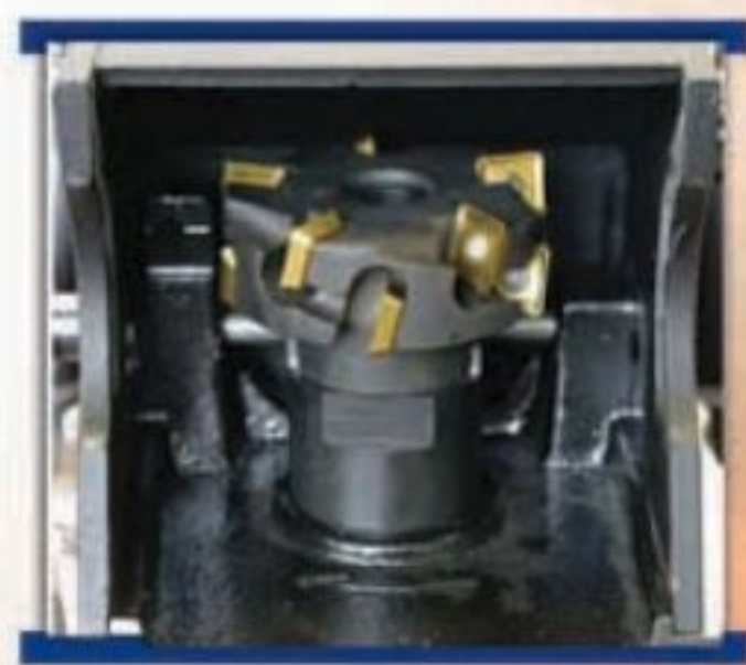
Mono block milling head, with 10 indexable inserts fixed with screws
